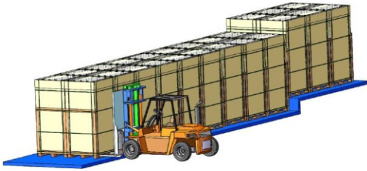
Vertical portrait package unloading with forklift
