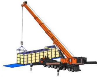
Vertical portrait package unloading with crane
