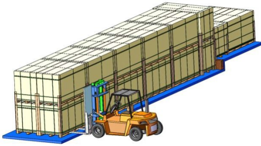
Vertical landscape package unloading with forklift
